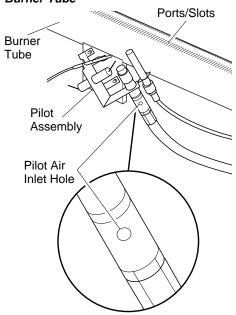
Figure 28 - Pilot Inlet Air Hole
